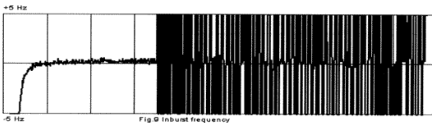
Figure 6a - switching on power amplifier disturbs frequency inside the burst
